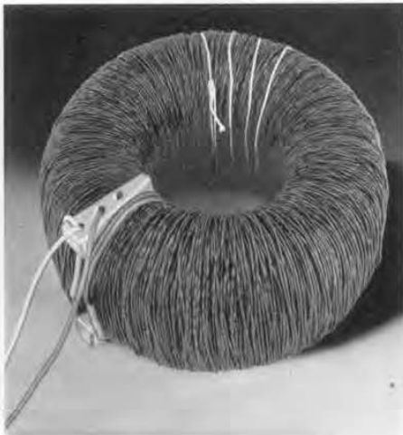
Figure 2. View of the toroidal inductor before installation in cabinet.
